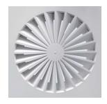
The standard TROX TCS/400 – 600 High-Flow Swirl Diffuser is designed to fit into different T-Bar ceiling patterns as well as plaster board ceilings and is available in either a square or a round face plate ranging from 400 x 400 to 600 x600 square or 400 Dia to 600 Dia. The diffuser has a radial airflow discharge pattern allowing for a high induction flow rate suitable for both variable and constant volume flow.
